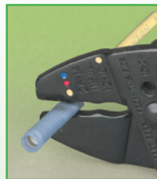
Make second crimp onto insulation
